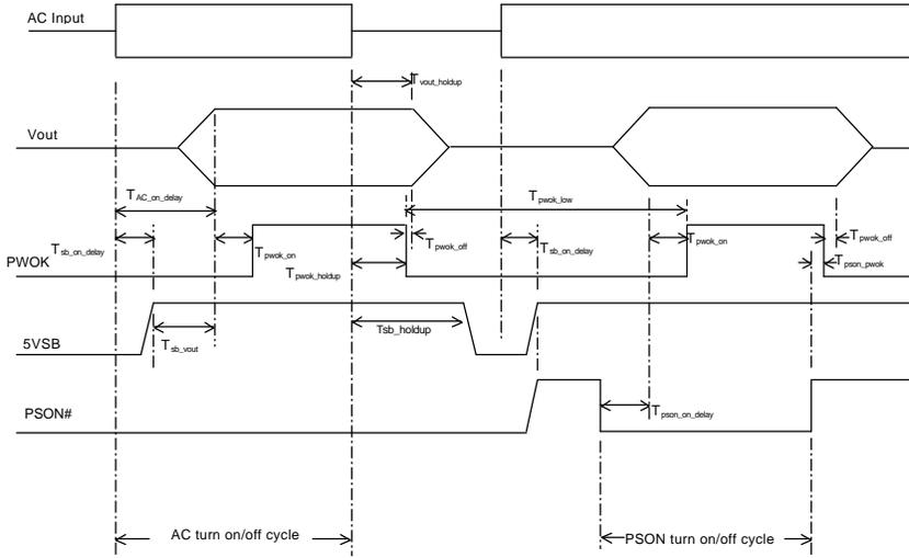
Figure 4: Turn On/Off Timing (Single Power Supply)
