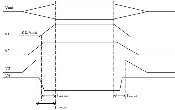
Figure 3: Output Voltage Timing
