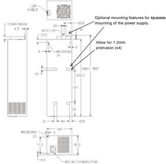
Figure 1: Enclosure Drawing
