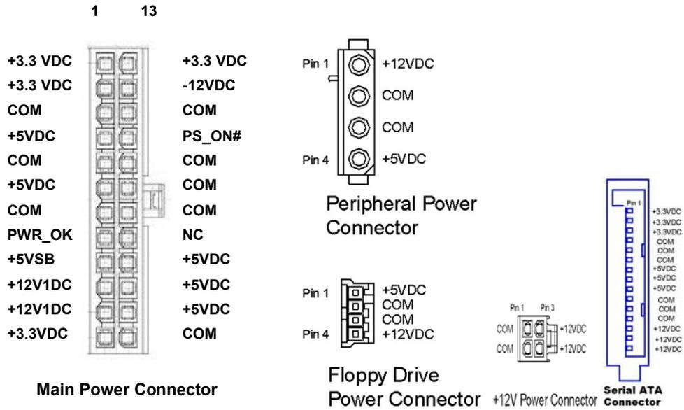
Figure 9. Connectors (Pin-side view, not to scale)
