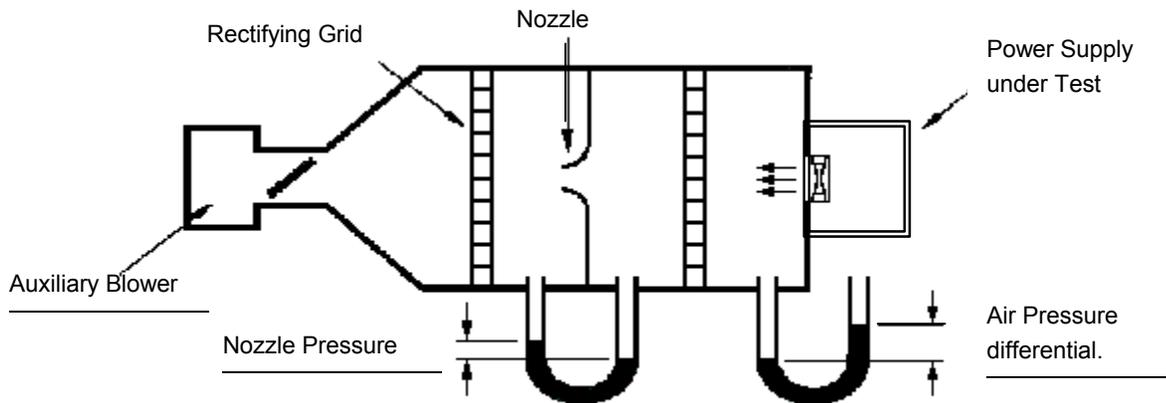
Auxiliary Blower is controlled to generate a zero Air Pressure differential. Air Flow is determined from Nozzle pressure.
