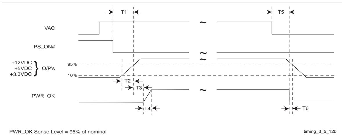
**Figure 5. Power Supply Timing**
