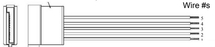
**Figure 10. Serial ATA connector**
